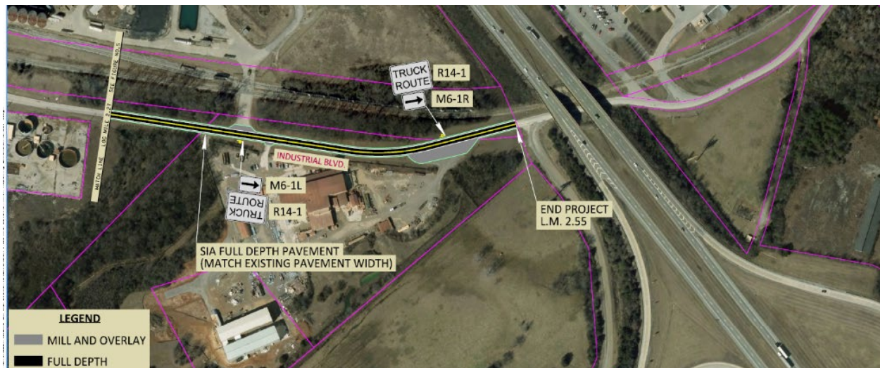
TDOT Design Concept (Marion County) – Phase 2 Improvements on Industrial Blvd. near I-24 underpass
