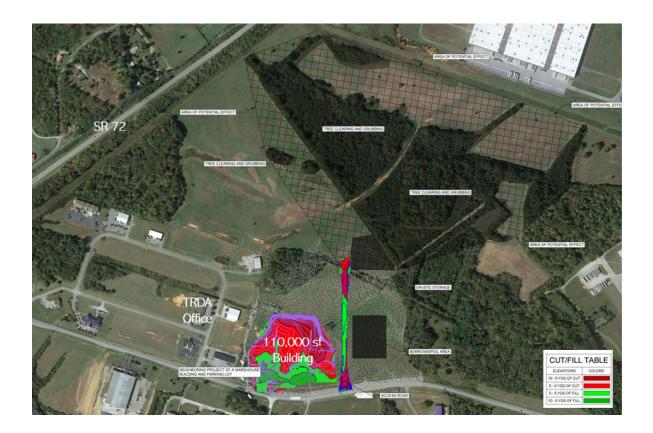
Like most construction projects, this one had its share of obstacles which included mid-project changes, utility relocation and the need for additional funding. TRDA had to relocate a 28-foot section of the 12-inch waterline. Once the road was cut to grade a new waterline was installed
